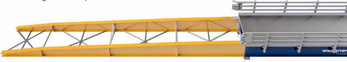
Beam bridge with launching nose
